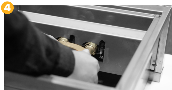
4 Gently pull and lift the Burner
