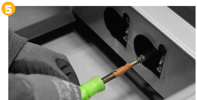
5 Use a 6mm socket to remove the NG orifice
