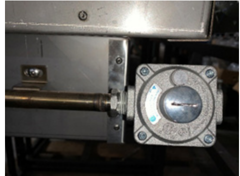
Step 3: LP gas "Hard Plumbed" conversion. Unscrew regulator cap.
